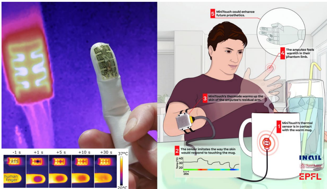
Left panel: an embodiment of the active thermal skin (ATS) sensor which allows to mimic temperature dynamics of the skin temperature (see insert). Right panel: example of an application of the thermal sensory feedback system applied to an upper limb amputee.
