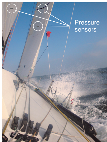
Fig. 1: A yacht equipped with wireless pressure sensors on luv and lee side. The connected solar cells enable independent wireless data transfer.
