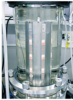
Biofilm reactor containing test coupons
